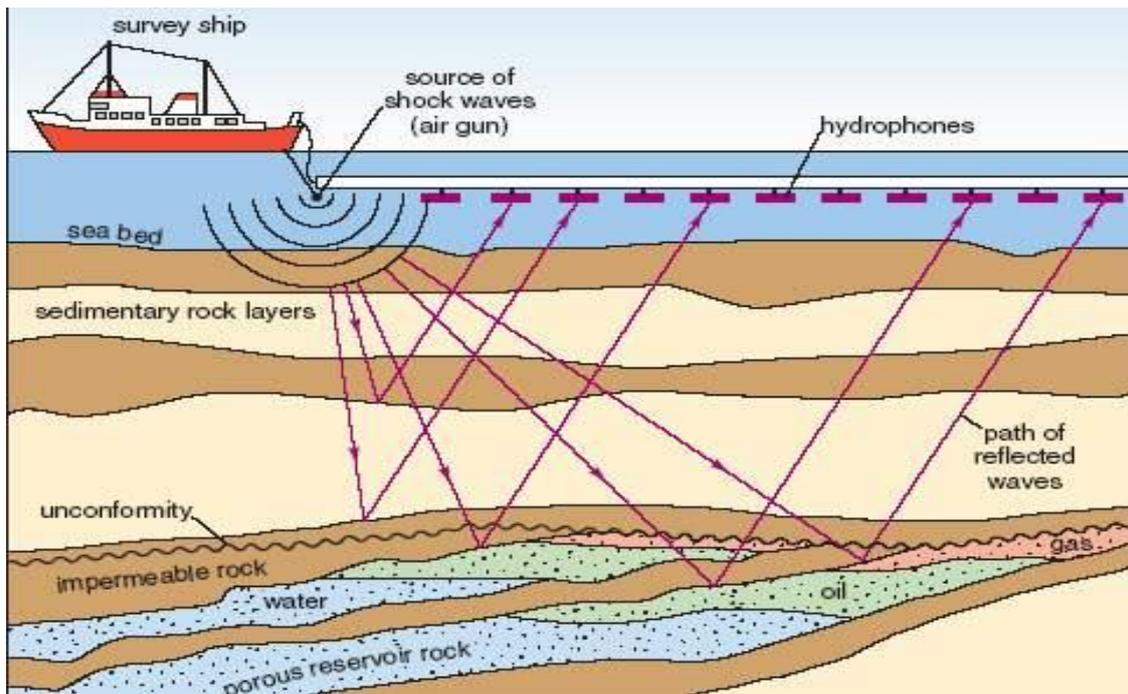
Figure 10. University Grants Commission (2015) *Offshore seismic survey scheme* In: *Oil and Gas Competency Building Workshop* p. 14
