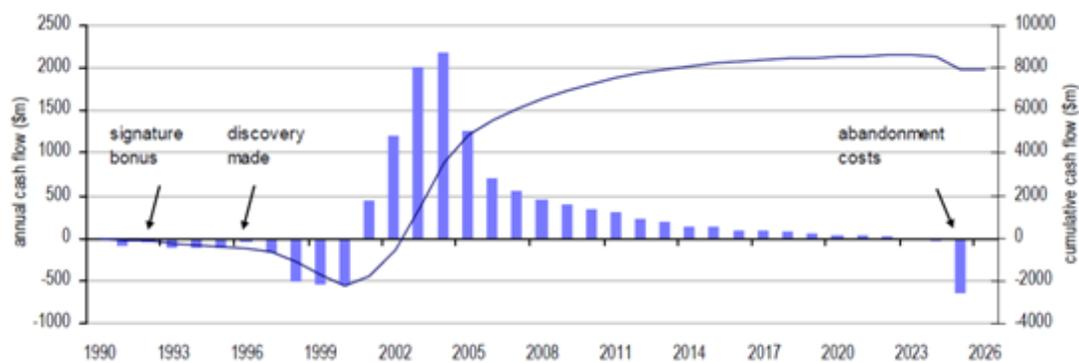
Figure 15. UBS Investment Research (2008) *Field life cycle example (Girassol field in Angola)*In: *Global Oil and Gas – Introduction to the oil industry* p. 84
