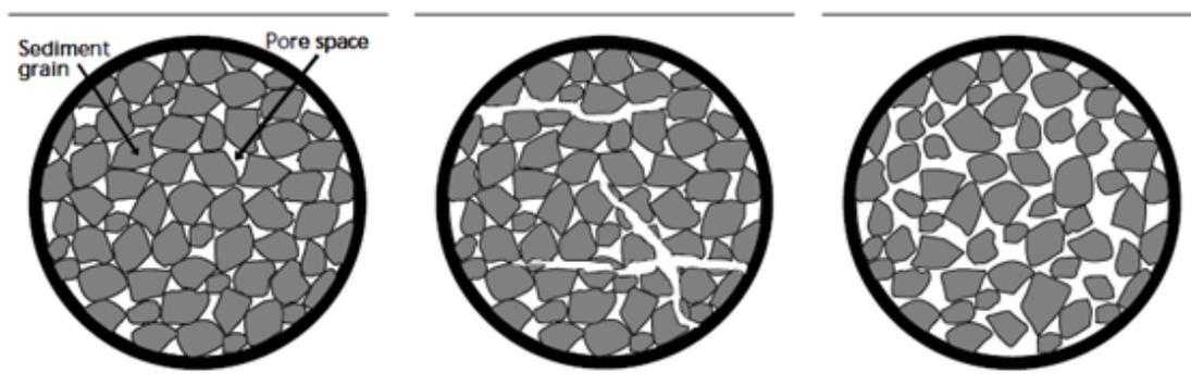
Figure 2. UBS Investment Research (2008) *Low porosity, low permeability* In: *Global Oil and Gas – Introduction to the oil industry* p. 80
